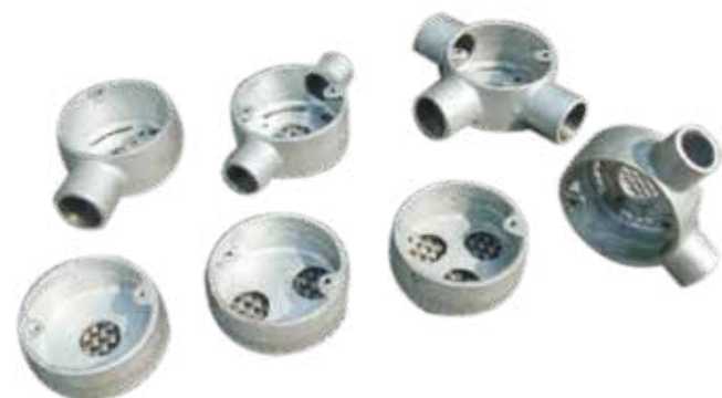
Malleable Iron Medium No. KB 272 Material: Malleable Iron. Finishes: Black Enamel, Galvanised. With tapped hole in base for earthing screw. 1,2,3,4Holes. Minimum: 31mm Deep X 63.5mm Inter.Dia.
